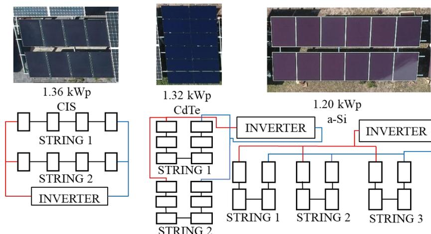
**Figure 1.** an Aerial image of the three thin-film PV arrays, together with a schematic of how they are connected. The peak output power of the arrays and the thin-film material of each array are also included.
