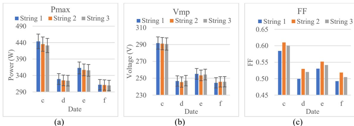
**Figure 8.** I-V curve parameters obtained for the 3 strings in the a-Si array.
