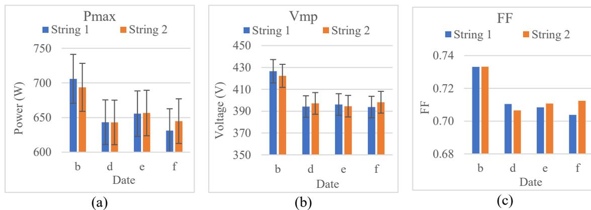
**Figure 7.** I-V curve parameters obtained for the 2 strings in the CdTe array.
